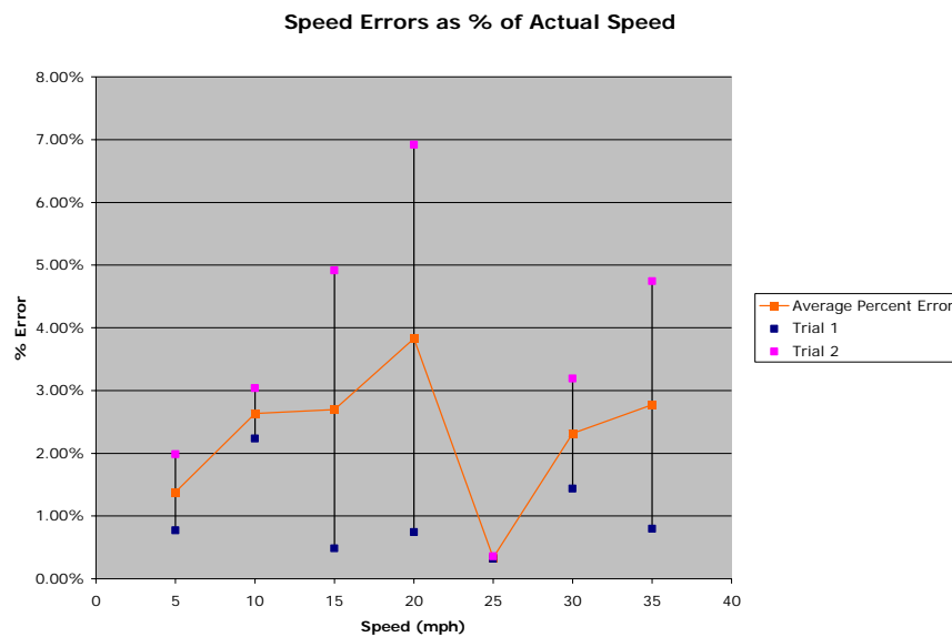
Figure 8.9 Sensys VDS240 Node and Internal Speed Percentage Error
